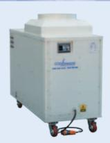
Model No. CB20000 Cooling Capacity 21.5kW **Power Supply** 415v/32a, 3-Phase **Current Consumption** 17.4a 3,060 Air Flow - Evap.m<sup>3</sup>/hr **Exhaust Duct Diameter** 500mm Exhaust Duct Length 10m (max) 73dB(A) Noise Level 740 x 1670 x 1212mm Dimensions (WxDxH) Weight 300kg Coverage 200m<sup>2</sup>
