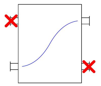
Another application where baffles aren't recommended is when you're using a buffer tank for storage. Here you would use a sparge pipe.
