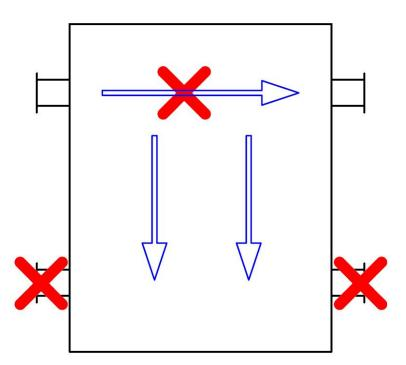
In this case, the majority of the tank is rendered useless, with the water that does travel downward moving at a different temperature and velocity to the water in the rest of the system, reducing efficiency.
